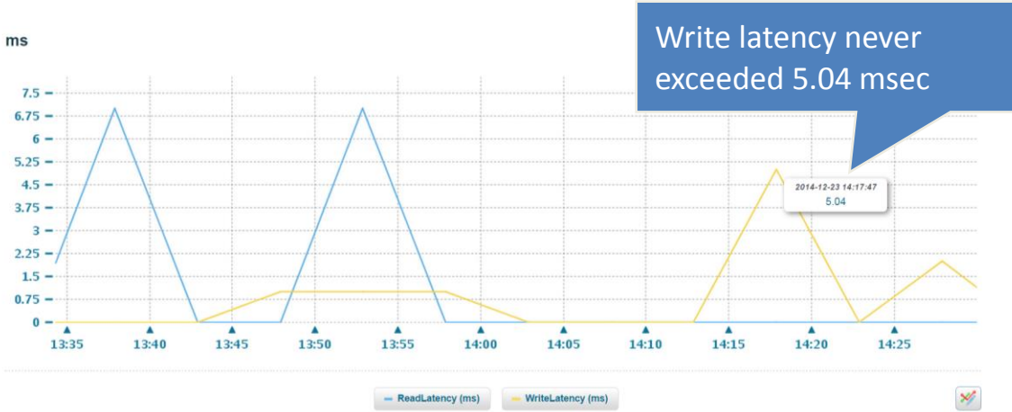
Figure 19. Write Requests & Write Latency results from SLA Reporting
